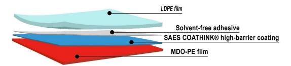
Figure 1 'Coathink®' technology by SAES Coated Films used as barrier coating
