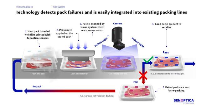
Figure 1. Senoptica HO3 technology by Senoptica used as responsive ink
